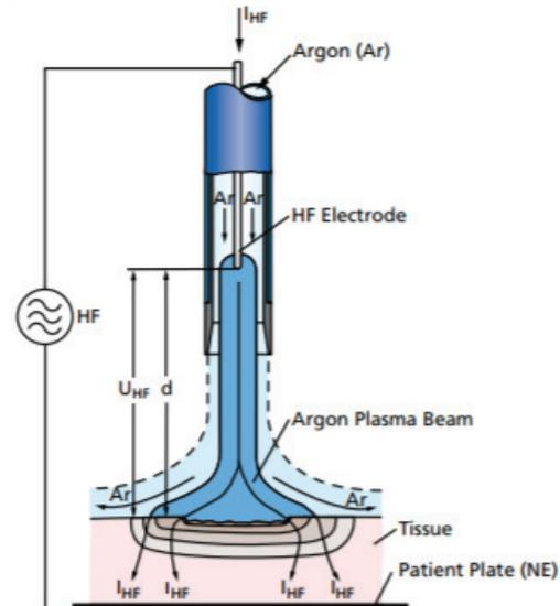
Transfer of energy from the APC probe to the tissue using ionized argon gas (argon plasma). HF = electro-surgical unit. IHF = high frequency/ electro-surgical current, UHF = high frequency voltage, d = distance between electrode and target tissue, Ar = argon, NE = patient plate
